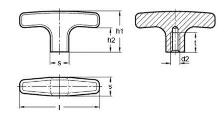
$\begin{array}{ll} d2 &= M6 \\ h1 &= 33 \\ h2 &= 22 \\ l &= 55 \\ s &= 14 \\ t min = 12 \end{array}$
